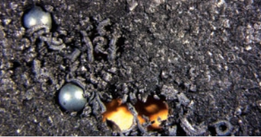
Comparison of spark protection: PyroGuard (top) Competitive Product (bottom)
